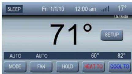
**Fig. 42 – Signal Strength Indicator Showing Good Strength**
