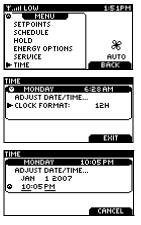
Press the Left Tab button on the home screen (MENU) to view this screen Use the SCROLL buttons to scroll to TIME menu. Press SELECT to enter the TIME menu.
