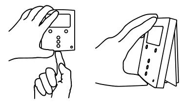
Warning: **do not use metallic tools** when removing battery or backplate; this may damage the thermostat.
