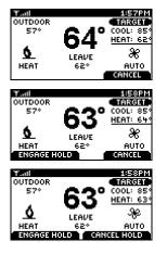
From the Home screen, press either of the *SCROLL* buttons to highlight the operating target SETPOINT (HEAT or COOL), which will be underlined.
