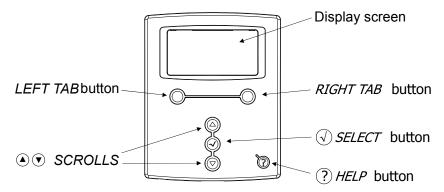
The function of the *LEFT* and *RIGHT TAB* buttons appears on the bottom of the display screen. Use the *SCROLL* ( $\blacktriangle \lor$ ) buttons to move through the menu items and options, and to change highlighted values. Press the *SELECT* ( $\checkmark$ ) button to select or accept highlighted menu items. You can always go back or cancel prior to saving changes.
