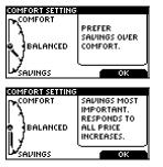
The **Savings** Comfort Level places a higher value on savings over comfort such that the temperature adjustments are greater for a given price increase.
